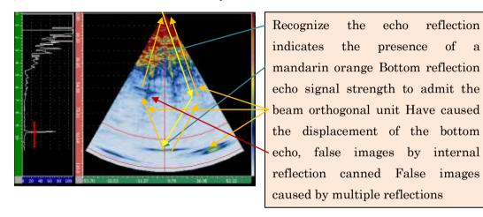
5MHz ultrasound image of an aluminum pack meat sauce HS-1500 in a manner similar equipment Recognize the reflected signal of the opposite side surface of an aluminum pack, inside the lesion characteristics, the observation of internal fluidity of the material was able to test at dynamic.
