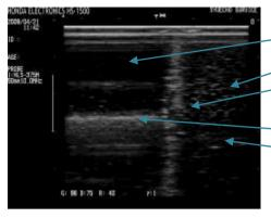
Clear, echo-free area of the water Gee nick echo area of the oil Boundary surface are shown in the left slope observed zonal high brightness, a cross-sectional findings 裂様. Wrap the bottom echo image bottled water Wrap oil bottle bottom echo image
